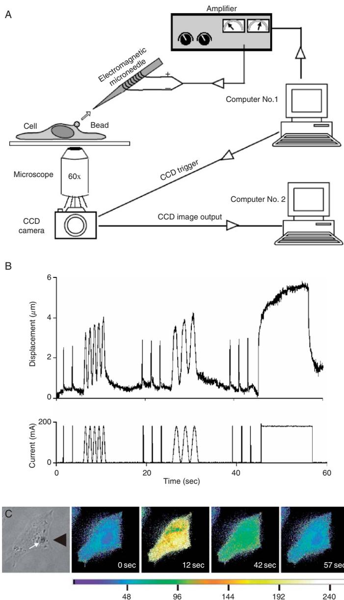
**Fig. 7** Electromagnetic pulling cytometry for analysis of cell mechanics and mechanotransduction. (A) Experimental system. A ligand-coated superparamagnetic bead is bound to receptors on the surface of a living cell, while a magnetic force (arrow) is applied to the bead using the electromagnetic microneedle. An amplifier supplies current to the electromagnetic microneedle and is controlled using LabVIEW on computer No. 1 to generate any arbitrary user-defined force regimen. The bead
