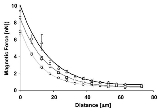
Fig. 2. Calibration of electromagnetic force acting on magnetic microbeads. The force acting on a 4.5  $\mu\text{m}$  diameter magnetic bead (Dyna) decreases as a function of distance from the microneedle tip and increases as a function of the electromagnetic current: 250 mA (circles, light gray curve); 500 mA (squares, dark gray curve) and 750 mA (triangles, black curves). At least 15 beads were analyzed for each value of the electric current (error bars indicate SEM).
