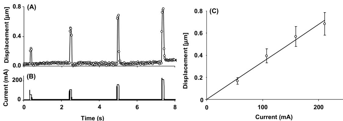
Fig. 4. Focal adhesions in living cells exhibit linear force–displacement behavior. (A) The measured bead displacement (○) during four 100 ms force pulses of increasing magnitude ( $\sim 100$  pN to 1 nN). (B) The electric current delivered to the electromagnetic microneedle corresponding to the displacement results shown in panel (A). (C) A plot of the maximum bead displacement as a function of electric current reveals a linear force–displacement relationship in the range of force investigated.
