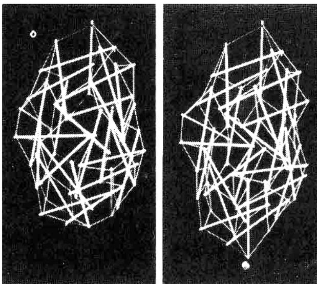
**Figure 3** : The discrete elements of a prestressed tensegrity structure composed of sticks and elastic strings undergo global rearrangements when a stress (metal weight) is applied to the lower vertex, as shown on the right.
